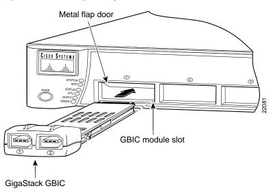
Figure 2-1 Inserting the GigaStack GBIC into a Switch Module Slot
